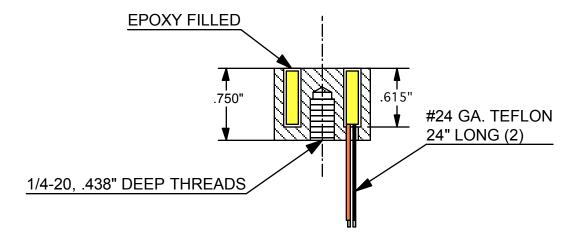
VOLTAGE: 12VDC CURRENT: 3.6 WATTS DUTY CYCLE: CONTINUOUS HOLDING POWER: 12 LBS
