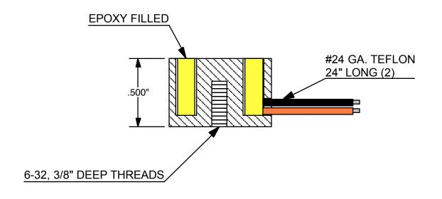
VOLTAGE: 24VDC CURRENT: 3 WATTS
