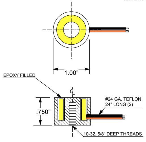
VOLTAGE: 24 VDC CURRENT: 3 WATTS
