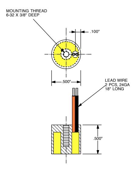
MODEL #: CE-050-12C VOLTAGE: 12 DC CURRENT: 3 WATTS
