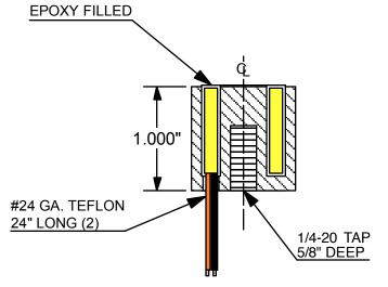
VOLTAGE: 12VDC CURRENT: 3.6 WATTS DUTY CYCLE: CONTINUOUS
