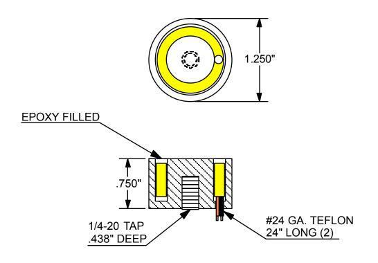
VOLTAGE: 12VDC CURRENT: 3.6 WATTS
