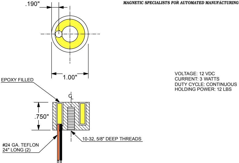
**VOLTAGE: 12 VDC CURRENT: 3 WATTS**
