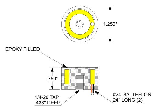
VOLTAGE: 24VDC CURRENT: 8.2 WATTS DUTY CYCLE: CONTINUOUS HOLDING POWER: 60 LBS
