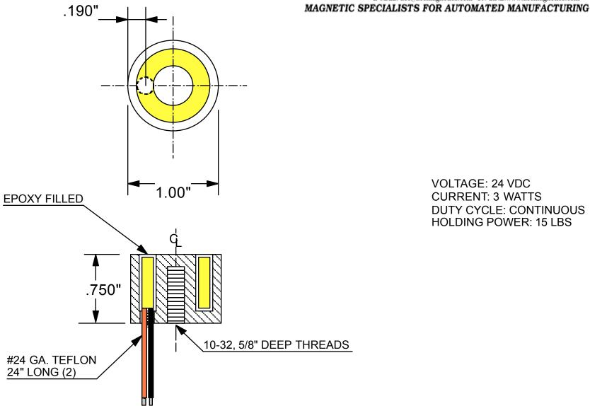
**VOLTAGE: 24 VDC CURRENT: 3 WATTS**
