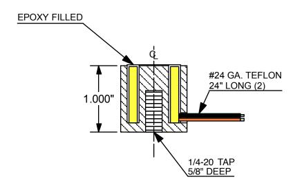
**VOLTAGE: 24VDC CURRENT: 8.2 WATTS DUTY CYCLE: CONTINUOUS**
