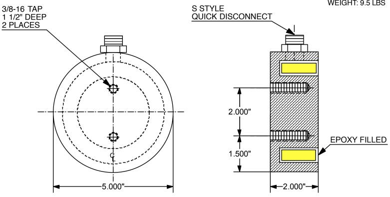
NITRIDING OXIDIZING PROTECTION ON ENTIRE MAGNET BODY TO PREVENT WEAR AND CORROSION
