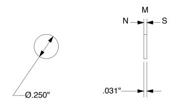
MATERIAL: 0.250" DIA X .03125" THK NEO 42 NICKEL PLATED & MAGNETIZED
