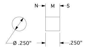
MATERIAL: 0.250" DIA X 0.250" THK NEO 42 NICKEL PLATED & MAGNETIZED
