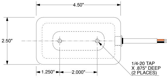
MODEL: EM-2545-24C VOLTAGE: 24VDC CURRENT: 26 WATTS
